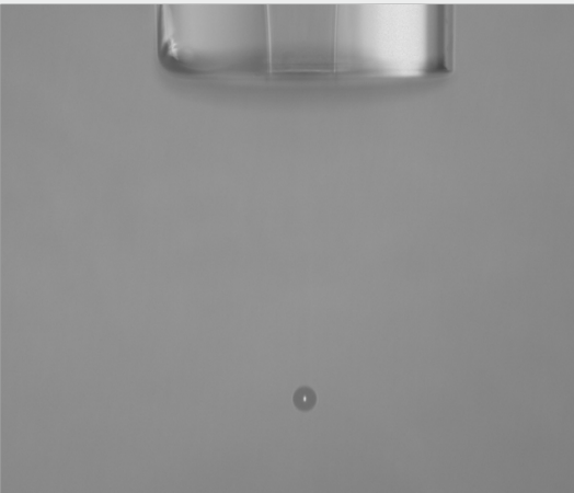
Figure 5: Average droplet diameter of AD-K-901 with inner nozzle diameter of 30µm showing different droplet sizes at different pulse settings. Note: Click on image to see a video of the droplet formation.
